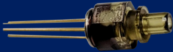
TOSA Transmitter Optical Sub-Assembly
